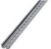
DIN rail perforated, Standard profile, width: 35 mm, height: 7.5 mm, acc. to EN 60715, material: Steel, Galvanized, white passivated, length: 2000 mm, color: silver
