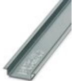
DIN rail, unperforated, Standard profile, width: 35 mm, height: 7.5 mm, acc. to EN 60715, material: Aluminum, uncoated, length: 2000 mm, color: silver
