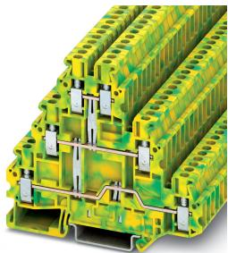
Ground modular terminal block, connection method: Screw connection, cross section: 0.14 mm<sup>2</sup> - 4 mm<sup>2</sup>, AWG: 26 - 12, width: 5.2 mm, color: green-yellow, mounting type: NS 35/7,5, NS 35/15
